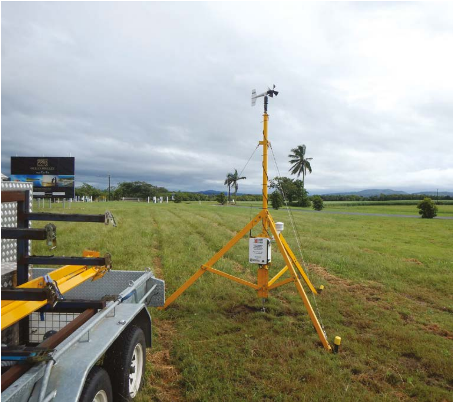
Cyclone Testing Station SWIRLNet anemometer, Cooktown: Portable wind station measuring wind speeds against Cyclone Ita 2014.
